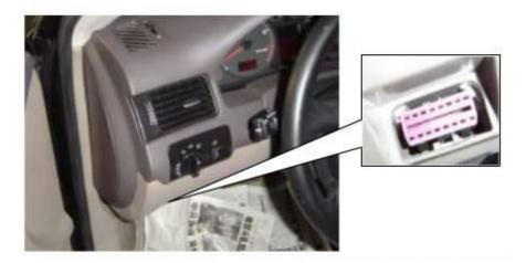
\*AUDI A6: the OBD plug is on the lower left side of the dashboard, use SMART OBDII-16 connector.
