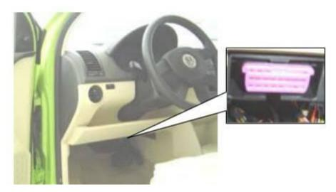
\*VW POLO: the OBD plug is below the dashboard, use SMART OBDII-16 connector.
