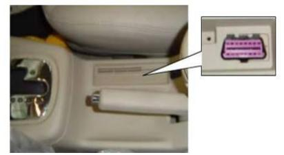
\*VW Passat B5: the OBD plug is behind the gearlever and beside the parking brake lever. Lift the cover to access it. Use SMART OBDII-16 connector.
