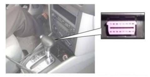
\*VW Bollywood 1.8: the OBD plug is below the console, use SMART OBDII-16 connector.
